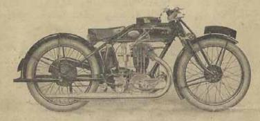
4'98 h.p. 3-SPEED A.J.S. OVERHEAD VALVE RACING MACHINE
