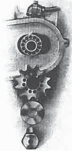
Magneto Timing—Vernier Adjustment.
