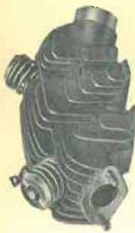
One of the new O.H.V. cylinder heads, the improved flange fitting to the carburettor will be noticed.
