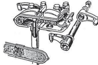
This sketch shows the design of the overhead rocker gear on 35/6, 35/18 and 35/8 Models. The rockers are duralumin forgings, attached by splines to the hollow alloy steel rocker spindles. Observe the ample diameter of the bronze bushes for the spindles and the neat manner in which the ball-ended duralumin push rods are enclosed.
