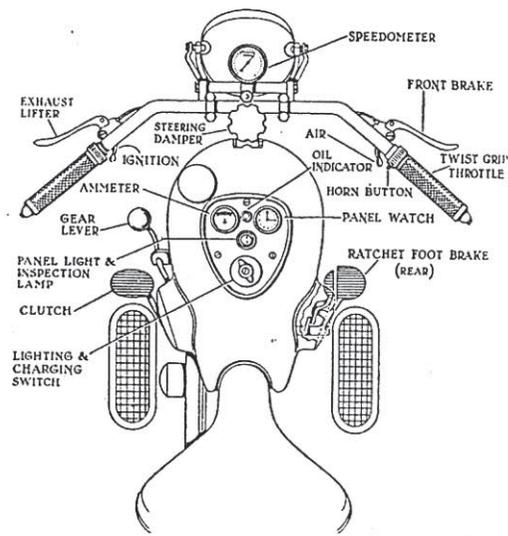
the twist grip, front brake, air control lever and horn button situated on the right handlebar. On the left handlebar will be found the exhaust lifter, ignition control lever and dipping and dimming device. The gear change lever is placed on the left-hand side of the petrol tank. The clutch is foot controlled by a pedal situated in front of the left footboard and the rear brake is controlled by a pedal in front of the right footboard. There is a ratchet locking device on the rear brake pedal.
