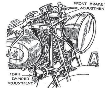
A well-known feature of "A.J.S." Motor Cycles is the exceptionally sturdy front fork assembly shown above. Note the accessible finger adjustment for the front brake, the convenient shock absorber adjusting knob, and the stiff headlamp mounting.
