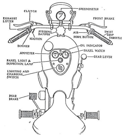
**CONTROL LAY-OUT.** The illustration on the left shows the English Control Lay-out on the Model 35/2.
