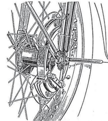
This cutaway view of the highly efficient front brake used on all Models except 35/12, 35/5, 35/16 and 35/4, shows the alloy drum with its cooling fins, which serve also to stiffen the drum to prevent distortion, the aluminium alloy brake shoes, and the neat manner in which the operating cable is concealed by passing through the front fork tube, whence it emerges at the finger adjuster shown in the top illustration.
