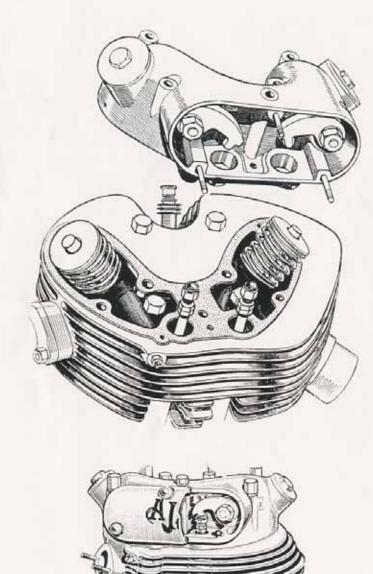
The illustration on the left shows the latest type of A.J.S. overhead valve gear, with the rocker box detached from the cylinder head to show the disposition of the valve springs and the push rods which operate the overhead valve rockers.
