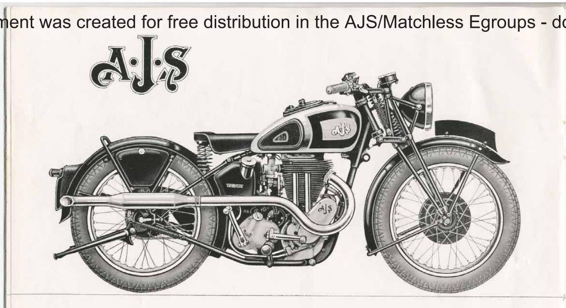
498 c.c. O.H.V. De Luxe Model. Single-port exhaust system. Petrol tank chromium plated with black panels lined silver and blue. Wheel rims chromium plated with silver centres and black lines. Sports mudguards. Check-spring front forks. (For full specification see pages 4 and 5.)
