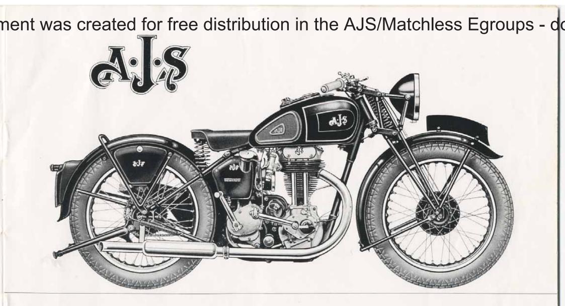
246 c.c. O.H.V. Standard Model. Coil ignition, single-port exhaust system. Petrol tank finished in black and gold. (For full specification see pages 4 and 5.)
