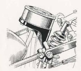
On all the "De Luxe "series and "Silver Streak "models, the speedometer is carried on the neat bracket shown in the illustration, the position being such that the rider can see the dial without removing his vision from the road ahead. This sectioned drawing shows clearly the dry-sump lubrication system of the A.J.S. Big Twin engine. A similar lubricating system is used on all 1939 A.J.S. engines, ensuring a constant and copious supply of cool clean oil to all working parts.
