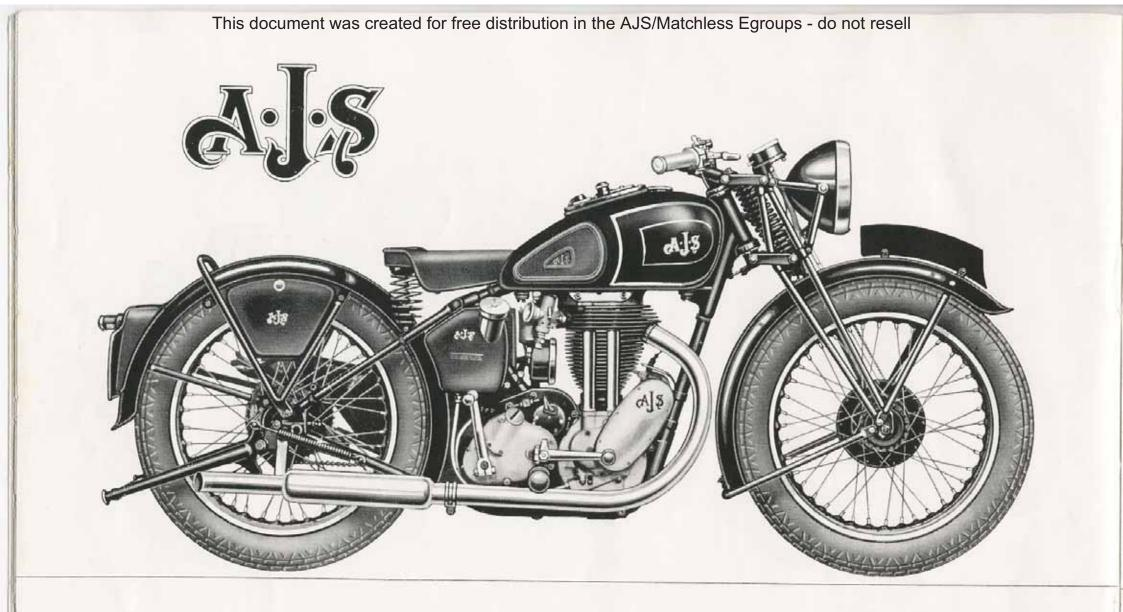
347 c.c. O.H.V. Standard Model. Magneto ignition, single-port exhaust system. Petrol tank finished in black and gold. (For full specification see pages 4 and 5.)
