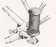
If a pillion passenger is to be carried, A.J.S. folding pillion footrests should be specified ( per pair). These fit into special lugs provided in the frame.
