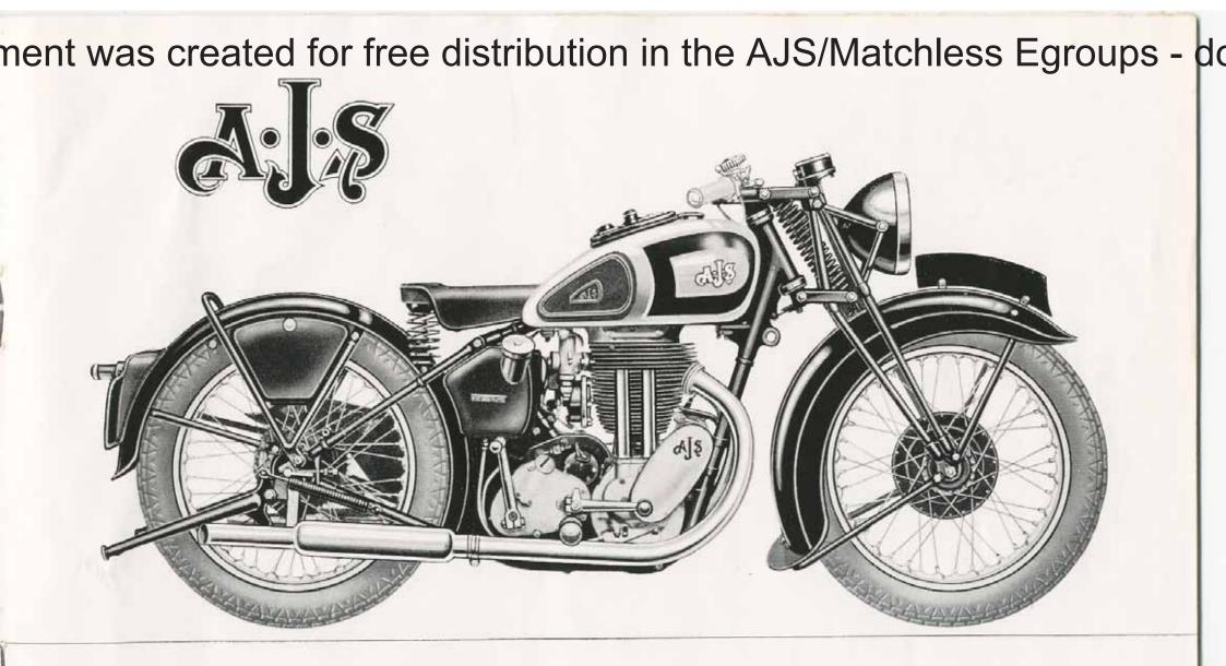
498 c.c. O.H.V. De Luxe Model. Two-port exhaust system. Petrol tank chromium plated with black panels lined silver and blue. Wheel rims chromium plated with silver centres and black lines. Valanced mudguards. (For full specification see pages 4 and 5.)
