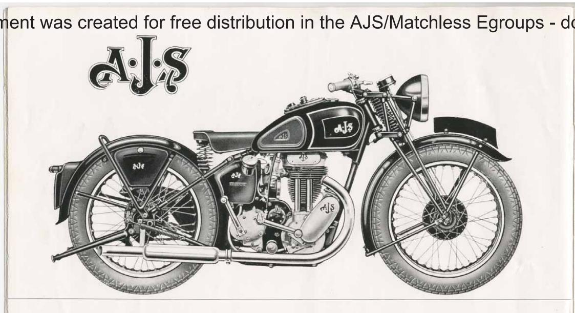
246 c.c. O.H.V. Standard Model. Magneto ignition, single-port exhaust system. Petrol tank finished in black and gold. (For full specification see pages 4 and 5.)
